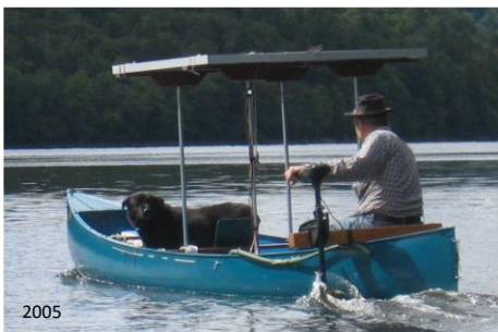
Figure 1. Converted solar electric propulsion canoe.
