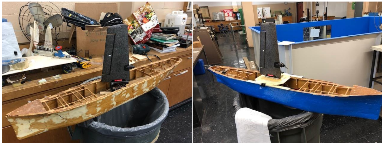
Figure 15. Ship Model before- and after full assembly. Figure at right shows remote controlled rudder and propeller. The aileron was not used in tests.
