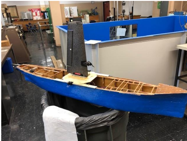
Figure 1. The Propeller Sail model with one propeller.
