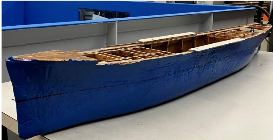
Fig. 1A. The USMMA ship model hull in its restored mode (painted hull and marked water line)
